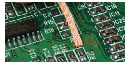
Match braid width to contact area
